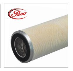
Series C coalescer cartridges are used in vertical and horizontal PECO Series 110 vessels and also as a retrofit to other competitor equivalents. The cartridge is designed to coalesce and separate free and entrained water from fluids such as aromatics, condensate, diesel, gasoline, kerosene, LPG and lube oil. The cartridge can also be used to remove entrained liquids other than water.
